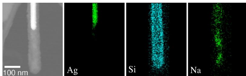
**Figure 2.** STEM study of S-SiO<sub>2</sub>-NWs following exposure to EPA medium. Left panel shows the STEM image; other panels show corresponding elemental maps depicting the distribution of silver (Ag), silicon (Si), and sodium (Na).
