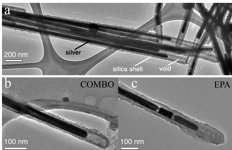
**Figure 1.** TEM study of the morphology of the aluminosilicate coating on (a) as-synthesized S-SiO<sub>2</sub>-NWs, or following a 2 h exposure to (b) COMBO or (c) EPA media. Other representative micrographs showing morphological changes in the S-SiO<sub>2</sub>-NW exposed to EPA media are given in Figure 2 and Figure S4.
